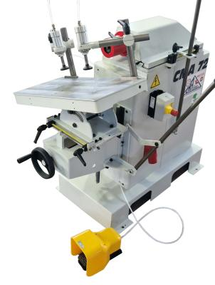
TILTING TABLE The revolving fence (goniometer) on the table -  $45\,^{\circ}$  / +  $45\,^{\circ}$  allows to perform any kind of work in full comfort and safety.
