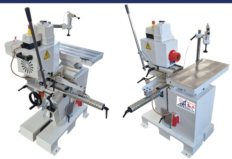
The CTM project (Cavatrice a Testa Mobile -Modile head bit mortising machine) has evolved, this model has always been characterised by its great rigidity, as the workpiece is on a fixed surface and the movements are operated by the drilling unit, this has always guaranteed an excellent workpiece processing. Today, the CTM EVO is equipped as standard with a tilting table and recirculating ball bearing guides.
