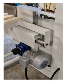
MOTORISED LIFTING OF THE WORK SURFACE The lifting of the work surface is motorised with a gear motor with high torque, allowing a linear and precise movement; only one lifting gear motor is provided as standard, but the machine can also be equipped with two gear motors for more heavy-duty work.
